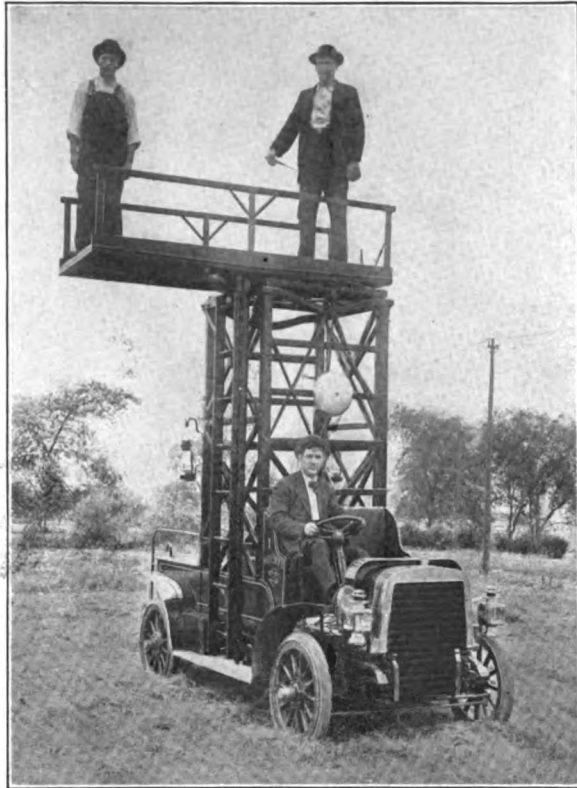
GASOLINE TOWER WAGON BUILT AND USED BY UNITED RAILWAYS COMPANY OF ST. LOUIS.
