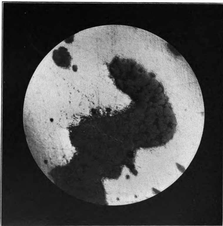
FIG. 10. SLAG IN IRON IN AN UNETCHED SPECIMEN.
