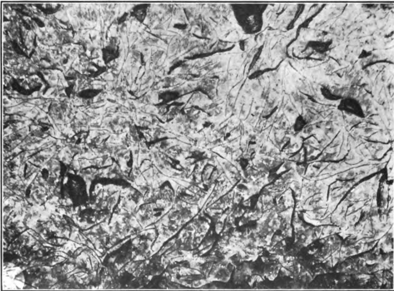
FIG. 12. CAST IRON SHOWING CARBON AFTER ANNEALING.
