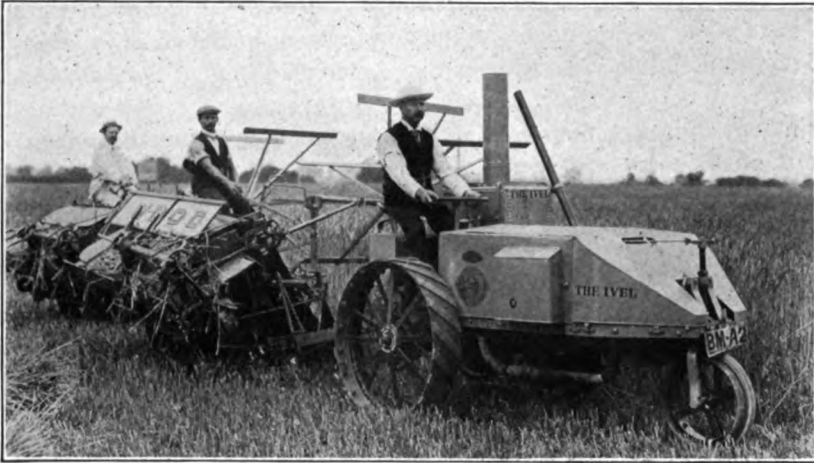
IVEL GAS-ENGINE AGRICULTURAL TRACTOR HAULING TWO REAPERS. Weight, complete, 3,584 lb.; engine, double-oppesed, 18-20 horse power, disposed longitudinally; consumes gasoline, kerosene, or alcohol.
