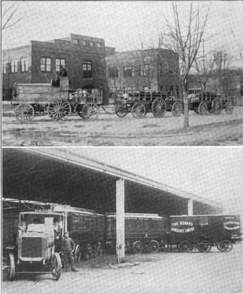
ABOVE, SAMPSON (AMERICAN) 20-TON ROAD TRAIN WITH ELECTRIC POWER TRANSMISSION; BELOW, RENARD (FRENCH) ROAD TRAIN WITH GASOLINE TRACTOR AND SIX-WHEEL TRAILERS.
