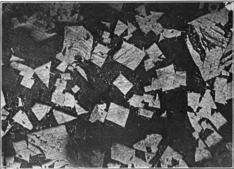
FIG. 11. ANTI-FRICTION METAL. Magnified 48 diameters.
